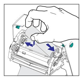
Before following these steps, prepare the ribbon by removing its wrapping and pulling its adhesive strip free.
