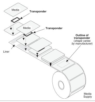
The communication between the RFID tag and the printer is established when the transponder lines up with the printer's antenna.
