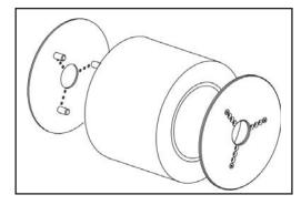
If your media roll has a larger diameter core, you can use an accessory to adapt the core to the media holders.
