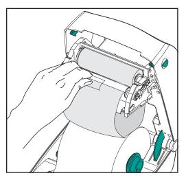
You must align the ribbon so that it will be taken straight onto the core.
