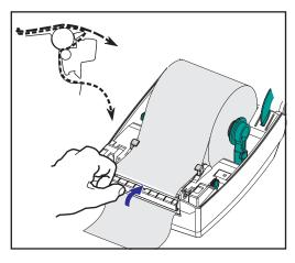
The optional dispenser allows you to print in "peel-mode" where the label backing follows a different path and the labels are presented one at a time for subsequent placement.
