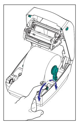
The adjustable guides direct the media toward the platen and print head.
