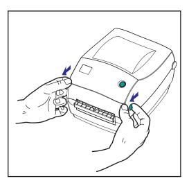
To access the media compartment, you must open the printer.
