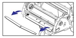
Before following the steps in this procedure, open the printer by pulling the release latches forward then lifting the top cover. Remove any ribbon from the carriage.
